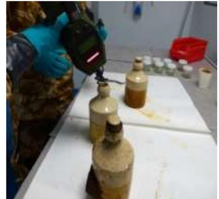
Pictures of the canisters, including testing for mustard gas at the analytical laboratory are included above (courtesy of Environment Agency, UK)
